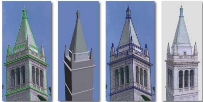
Original photograph with marked edges Recovered model Model edges projected onto photograph Synthetic rendering
