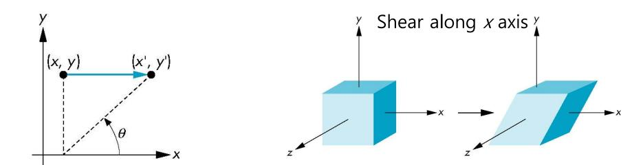
$$\begin{aligned} x' &= x + y \cot \theta \\ y' &= y \\ z' &= z \end{aligned} \mathbf{H}_{xy}(\theta) = \begin{bmatrix} 1 & \cot \theta & 0 & 0 \\ 0 & 1 & 0 & 0 \\ 0 & 0 & 1 & 0 \\ 0 & 0 & 1 & 0 \\ 0 & 0 & 0 & 1 \end{bmatrix} \\ \tan \theta &= \frac{y}{x' - x} \Rightarrow \cot \theta = \frac{x' - x}{y} \end{aligned}$$
