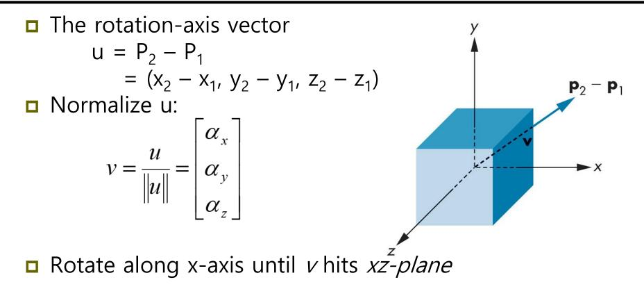
Rotate along y-axis until v hits z-axis
