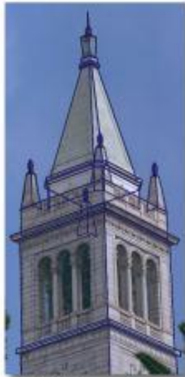
Model edges projected onto photograph
