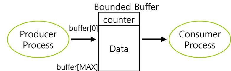
Producer writes new data into buffer and increments counter
