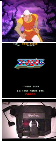
Vectrex 3D imager (uses CDRom drive to shutter glasses in synch with Vectrex screen)
