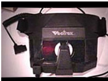
Vectrex 3D imager (uses CDROM drive to shutter glasses in synch with Vectrex screen)
