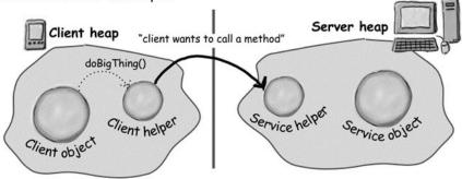
3 Service helper unpacks the information from the client helper, finds out which method to call (and on which object) and invokes the <u>real</u> method on the <u>real</u> service object.
