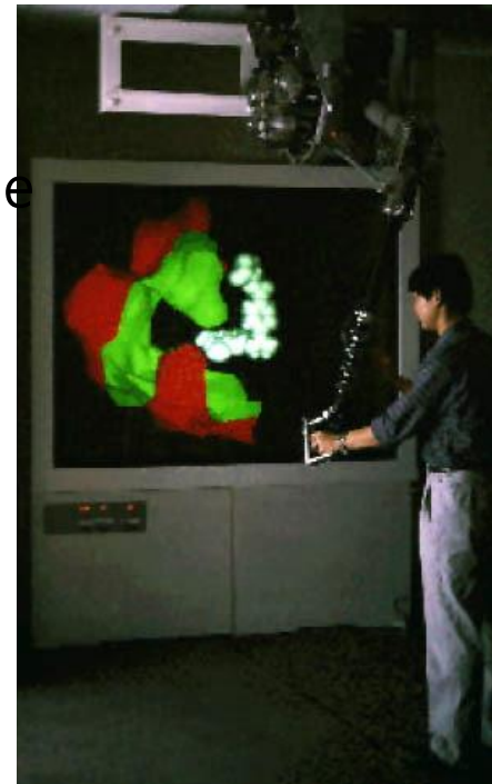
UNC's GROPE II 6-DOF ceiling mounted ARM (Argonne Remote Manipulator)
