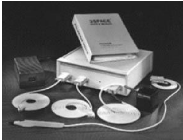
Polhemus FASTrak and VISIONTrak tracking system
