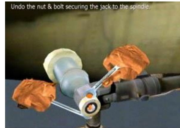
Maelstrom's virtual toolkit teaches technicians how to perform repairs to the Puma helicopter. Immersive tools – headset, cyber gloves, and Ascension's three sensor Flock of Birds – are used to simulate real-world conditions in which repairs often take place. Image courtesy Maelstrom Virtual Productions
