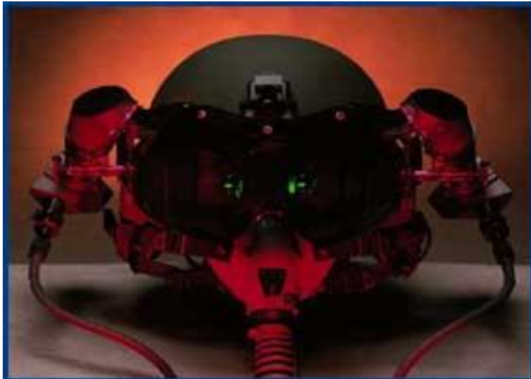
Figure 3: Virtual retinal display technology is being incorporated in helmet-mounted displays for military applications. (Photo courtesy of Microvision).
