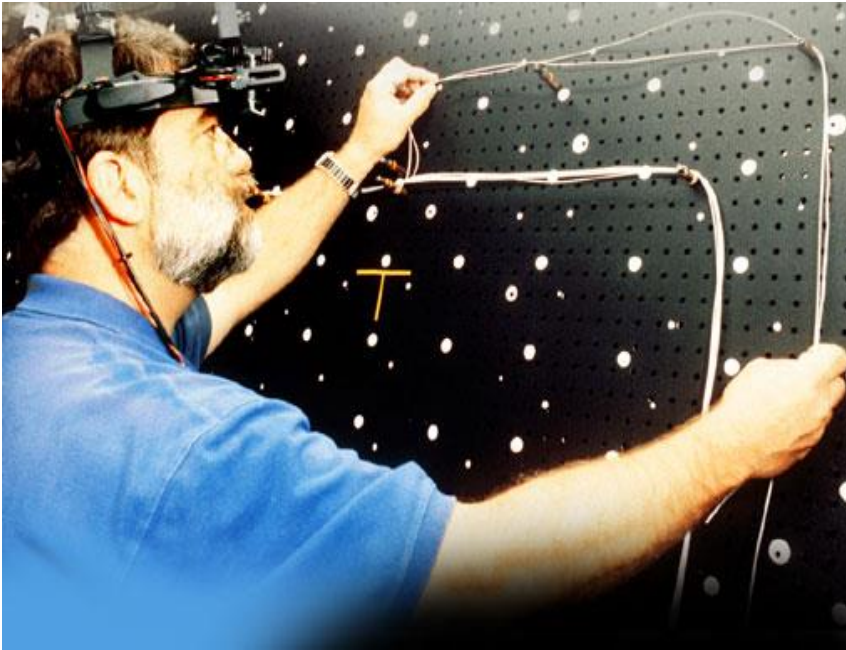
Layout Diagrams for the wire bundles appear “superimposed” on the layout board
