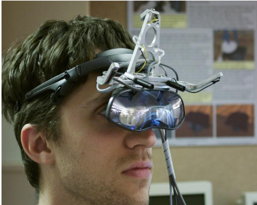
Video See-through Augmented Reality HMD built on the basis of a Sony Glasstron LDI-D100 device
