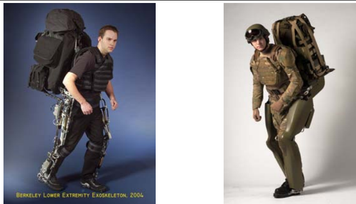
The BLEEX project, UC Berkeley, a self-powered exoskeleton, provides a versatile transport platform
