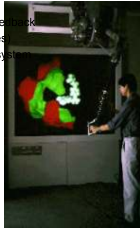
UNC's GROPE II 6-DOF ceiling mounted ARM (Argonne Remote Manipulator)
