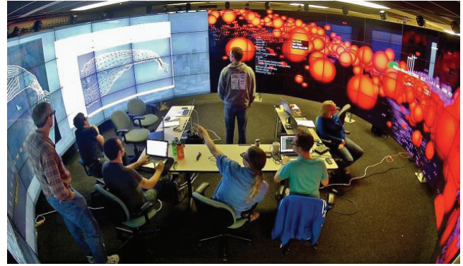
Fig. 5. Two photographs taken during a co-located collaborative meeting in CAVE2. On the left, an Omegalib immersive visualization is running on the full display. On the right, CAVE2 is split into two workspaces to display additional 2D views. Switching between the two modes can be done at runtime, without resetting running applications.
