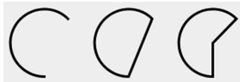
(a) Arc2D.OPEN (b) Arc2D.CHORD (c) Arc2D.PIE
