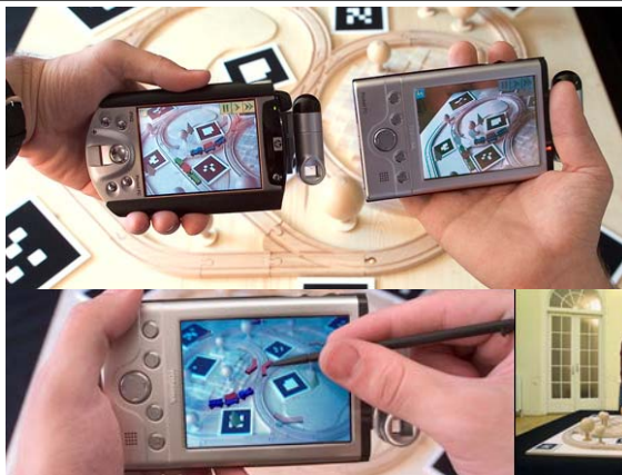
The Invisible Train @ Vienna University of Technology, Real-time multi-user augmented reality application for handheld devices
