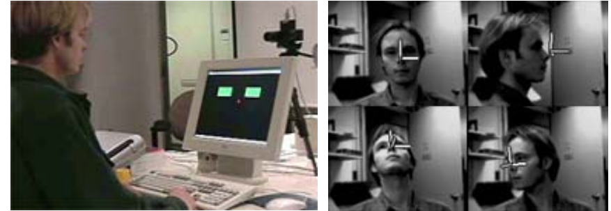
WATSON @AI Lab, MIT: Real-time head pose estimation using a stereo camera to recover the 3D rotation and translation of objects, or of the camera itself.
