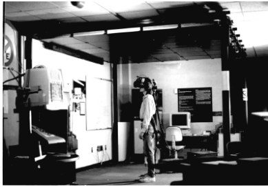
HiBall Tracker @ UNC uses image-sensing devices mounted on user's head
