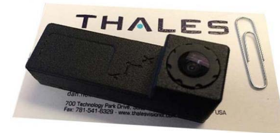
InterSense IS-1500, 6DOF Inertial-Optical Self-Tracking System for mixed reality and GPS denied navigation http://www.intersense.com/pages/70/255
