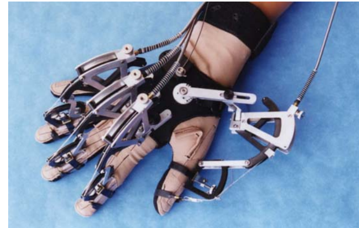
Virtual Technologies Inc, CyberGlove – tactile feedback, gesture, position & orientation tracking
