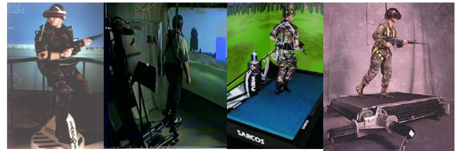
Sarcos Inc. Uniport, Biport, Treadport, Onmiport Displays unilateral constraints, inertial forces, and slope
